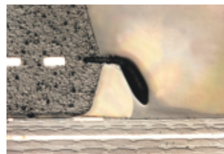
Cross section of an electronic part (coaxial illumination)
